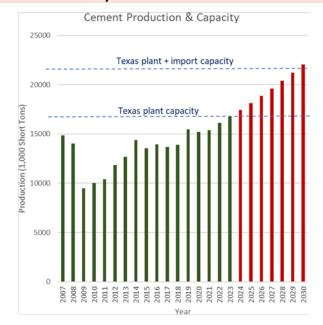
Texas produces more than 1.5 million tons of cement each year. Texas plant capacity is about 1.7 million tons and projected to be exceeded by 2024. Texas plant capacity and imports are expected to be surpassed by 2030 at current production and import rates.
