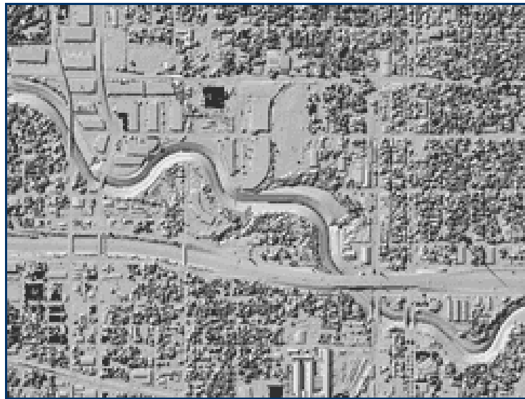
Image of White Oak Bayou near I-10, produced from LIDAR data.
